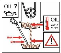
Checking the lubricating oil level.
