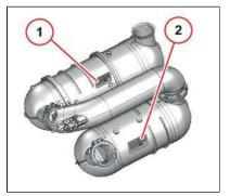
Serial numbers of the exhaust aftertreatment components
