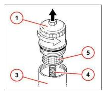
Replace lubricating oil filter cartridge
