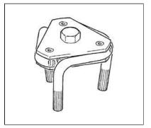
Special wrench for loosening exchangeable filters
