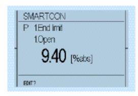
During operation, the displays shows the position of the actuator as a percentage, operation mode and status. When using the option identification, a customer-specific label is shown at the bottom of the display (e.g., PPS Number).
