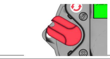
Figure 27 Selector Switch in Neutral Position (6)
