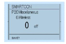
Thereafter, flip up the control switch toward to change the value from 0 (off) to 2 (Bluetooth).
