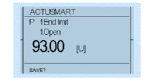
In order to confirm the end position (save), slightly flip up the selector switch and let it snap back to its neutral position.
