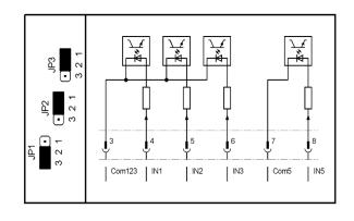
Jumpers JP1 to JP3 can be used to interconnect the binary inputs to groups with separate earths:
