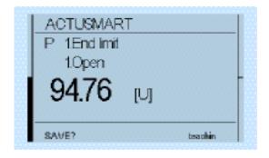
Manually move the actuator with the handwheel (see Section 13.1 or Section 13.6) or by motor via the operating switch (black button) to the end position OPEN of the valve.
