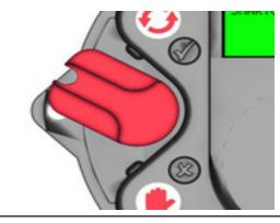
Figure 17 Selector Switch in Neutral Position (2)
