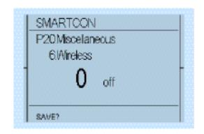
Use the control switch towards to the characters to change the parameter  $\oplus$  or  $\bigcirc$  (see Figure 42 to Figure 45). After reaching the desired parameter value, confirm the value with the selector switch again, flip it slightly towards  $\heartsuit$ , (see Figure 33 to Figure 35).
