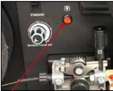
(13) Press and hold the inch wire button to feed the wire down the torch cable through to the torch head.
