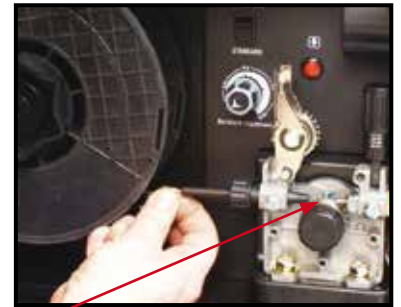
(12) Place aluminium wire onto spool holder. Feed the wire through and over the drive roller into the inlet guide tube.
