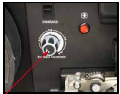
(17) Adjust the burn back control to prevent the wire sticking in the weld pool.
