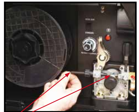
(7) Place wire onto spool holder - (spool retaining nut is left hand thread ) Feed the wire through the inlet guide tube on to the drive roller.
