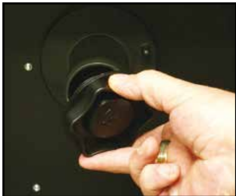
(1) Remove the spool retaining nut.
