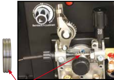
(11) Install a U groove drive roller of the correct size for the diameter wire being used.
