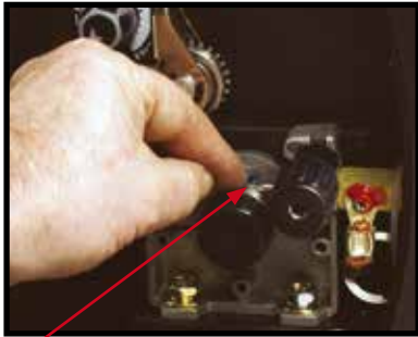
(8) Feed wire over the drive roller into the outlet guide tube, Push the wire through approx 150mm. Use a Knurled Drive Roller of the correct size NOTE: VIPER 182 not geared
