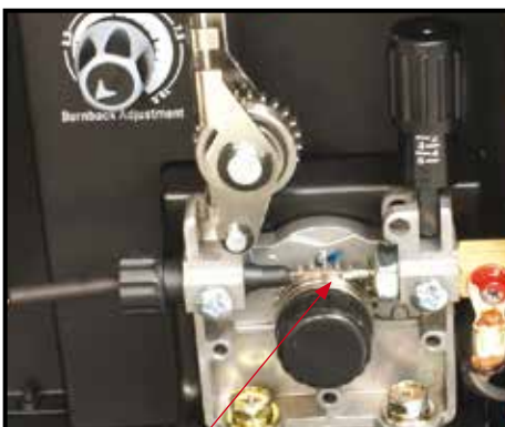
(5) Feed the wire through the drive roller and into the outlet guide tube of the wire feeder. NOTE: VIPER 182 not geared
