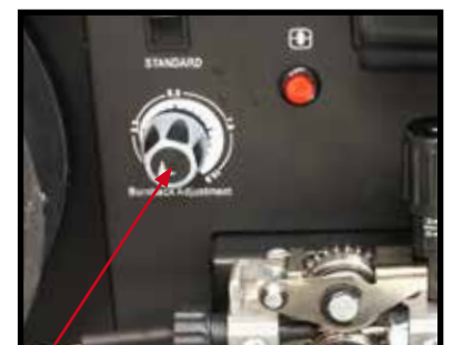
(16) Adjust the burn back control to prevent the wire sticking in the weld pool.
