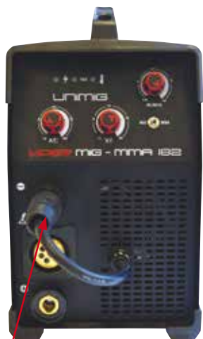
(2/5) Connect weld power lead to ⊖ negative terminal
