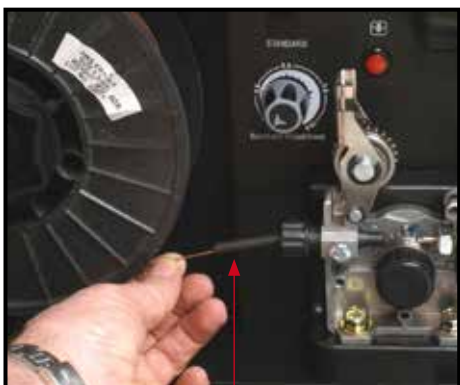
(4) Snip the wire carefully, be sure to hold the wire to prevent the spool uncoiling. Carefully feed the wire into the inlet guide tube of the wire feed unit.
