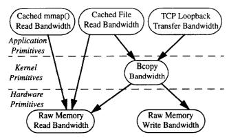
Figure 2: Decomposition of Application Data-access Primitives. All of the application-level data primitives for bulk data access depend on the hardware's memory read bandwidth since they all touch data. File reading interposes the extra overhead of a cross-protection-domain bcopy to move the requested data to user-space buffers; TCP transfer interposes three bcopy's as it shuffles the data through the loopback interface and between user and kernel space.
