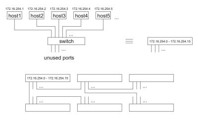
Figure 2.6: Above: a one-switch network, below: a uniform network
