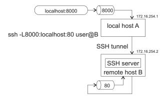
Figure 2.17: Local port forwarding over SSH with no unencrypted connections
