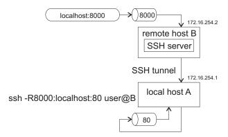
Figure 2.19: Remote port forwarding over SSH with no unencrypted connections
