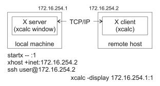
Figure 3.3: Starting an X client on a remote host
