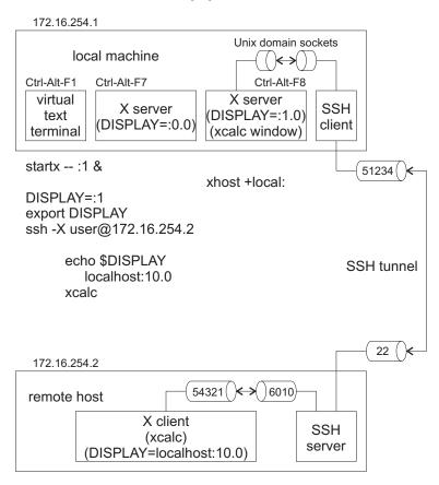
Figure 3.5: X11 port forwarding over a secured SSH tunnel
