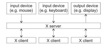
Figure 3.1: Client-server model of the X window system
