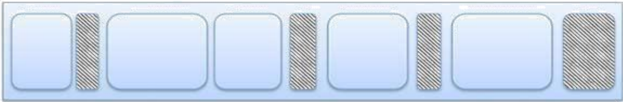
Fragmented memory before compaction
