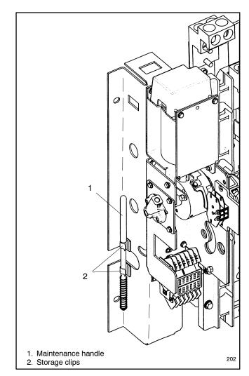
Figure 2-8 Manual Handle Storage, 600–1200 Amp Switch Shown
