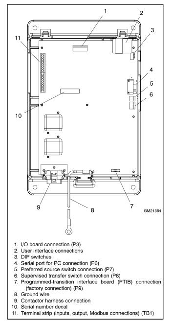
Figure 3-6 Controller Board Component Locations
