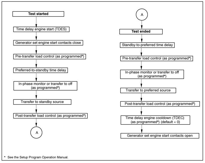
Figure 4-5 Test with Load Sequence
