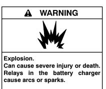
Locate the battery in a well-ventilated area. Isolate the battery charger from explosive fumes.
