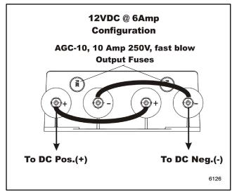
Figure 6-22 12-Volt Battery Charger Connections
