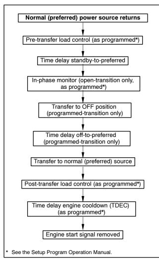
Figure 4-2 ATS Sequence of Operation, Return to Normal (preferred source)
