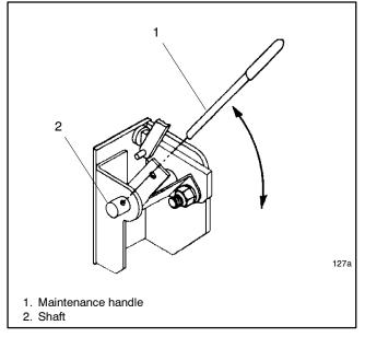
Figure 2-9 Manual Operation, 225-400 Amp Open-Transiton Switches and 150-400 Amp Programmed-Transition Switches (one operator shown)
