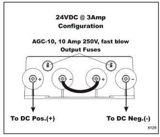
Figure 6-23 24-Volt Battery Charger Connections
