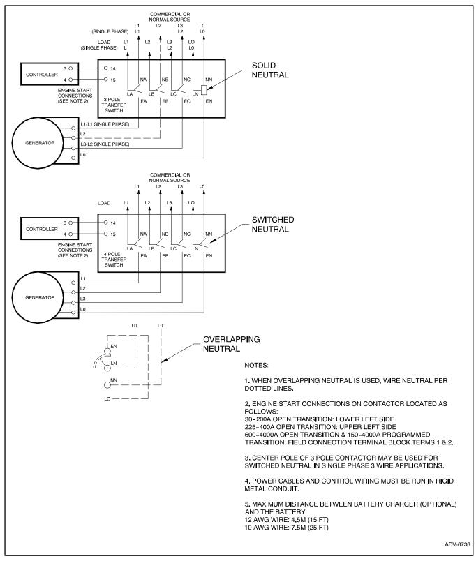
Figure 2-20 Interconnection Diagram
