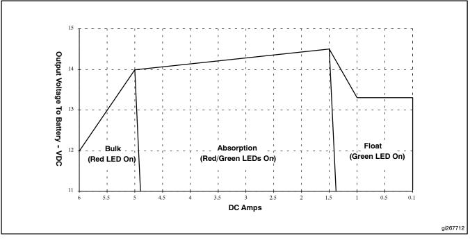
Figure 6-25 Charging Method, 12 VDC, 6 A Configuration
