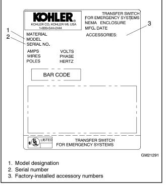
Figure 1-2 Typical Transfer Switch Nameplate
