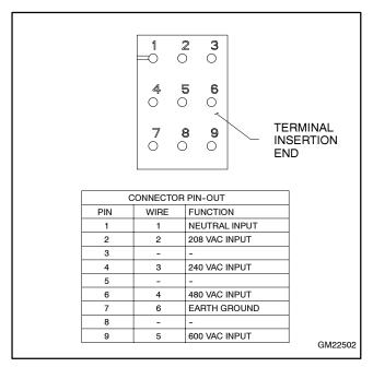
Figure 6-20 Battery Charger Power Connection
