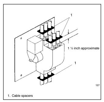
Figure 2-16 Cable Spacers for 30-200 Amp Switches
