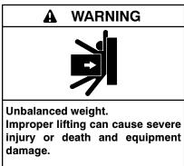
Use adequate lifting capacity. Never leave the transfer switch standing upright unless it is securely bolted in place or stabilized.
