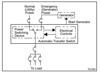
Figure 1-1 Typical ATS Block Diagram
