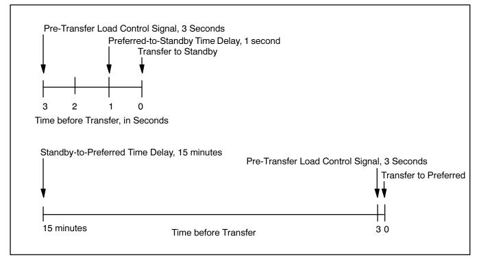
Figure 4-13 Pre-Transfer Time Delay Operation (default settings)
