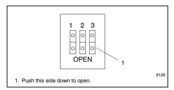
Figure 6-17 I/O Module Address DIP Switches
