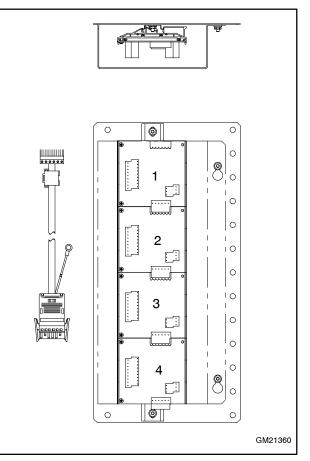
Figure 6-9 Input/Output Modules and Harness (cover is shown transparent to show detail)
