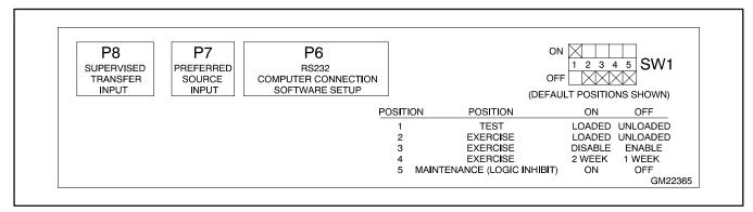
Figure 3-8 Logic Assembly Decal Showing DIP Switch Settings
