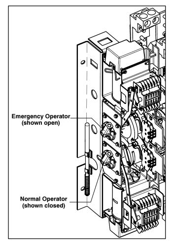
Figure 2-13 Programmed-Transition Switch Normal and Emergency Operators, 600–1200 Amp Model (shown in Normal position)
