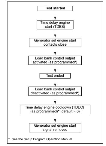
Figure 4-4 Test Without Load Sequence
