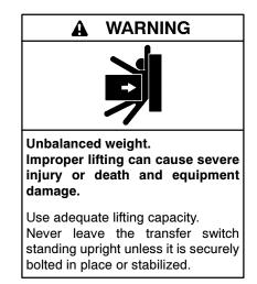
See Figure 2-1 through Figure 2-4 or the dimensional drawing for the weight of the transfer switch. Use a spreader bar to lift the transfer switch. Attach the bar only to the enclosure's mounting holes or lifting brackets; do not lift the unit any other way. Close and latch the enclosure door before moving the unit.
