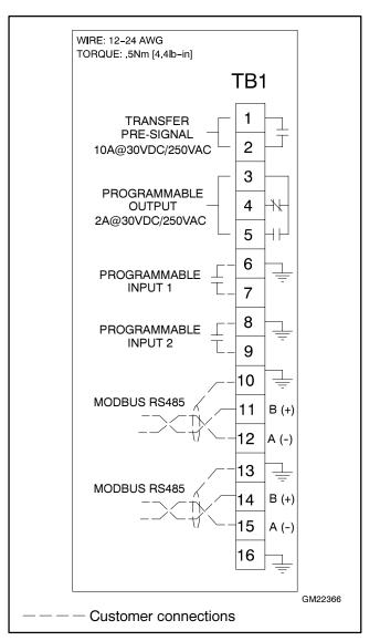
Figure 3-9 Terminal Strip TB1 Connections
