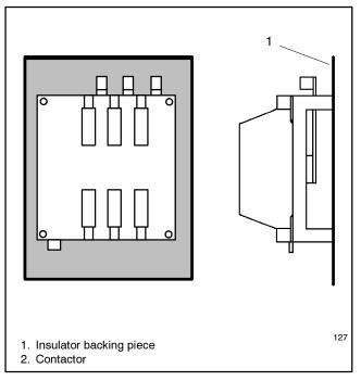
Figure 2-17 Insulator for 225-400 Amp Switches
