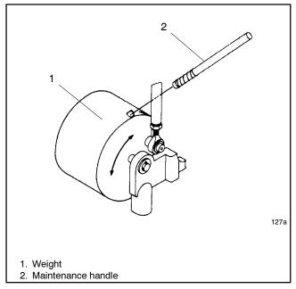
Figure 2-12 Manual Operation, 4000 amp switches
