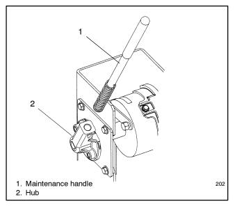
Figure 2-10 Manual Operation, 600–1200 Amp Switches
