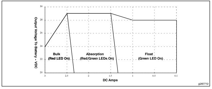
Figure 6-26 Charging Method, 24 VDC 3 A Configuration
