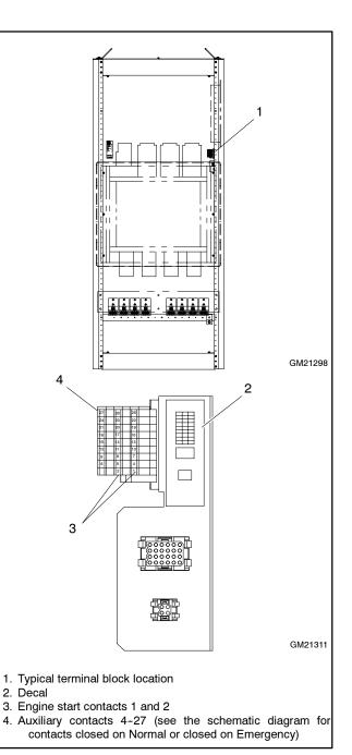
Figure 2-23 Engine Start and Auxiliary Contact Terminal Block, Programmed-Transition Models and 600–4000 Amp Open-Transition Models
