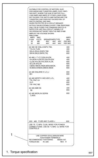
Figure 2-19 Typical Rating/Torque Label
