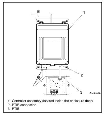
Figure 3-10 Programmed-Transition Interface Board (PTIB)
