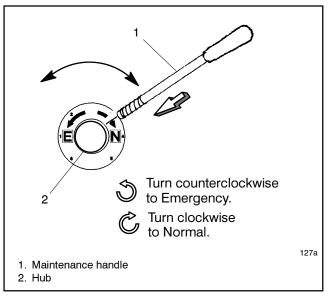
Figure 2-11 Manual Operation, 1600-3000 Amp Switches
