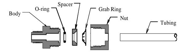
Step 1: Dissemble fitting components
