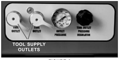
FIGURE 6 OPTIONAL TOOL OUTLETS P/N 805827-SERIES
