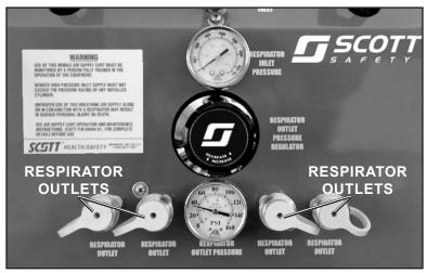
FIGURE 5 RESPIRATOR OUTLETS (FOUR OUTLET VERSION SHOWN)
