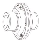
recommended. Sizes 1020T to 1090T20 are furnished with a pre-measured amount of grease for each coupling. The grease can be ordered for larger size couplings.
