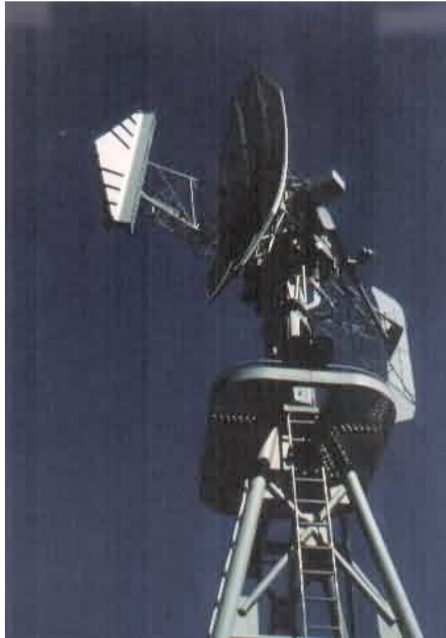
AN/SPS-8 – this radar “nodded” up and down
