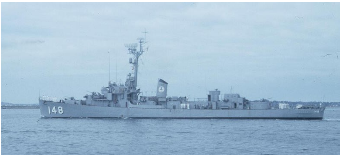
USS Brough 1956 – thicker foremast and updated radars
