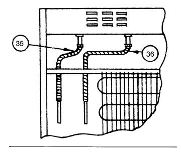
NOTE: Use pipe joint compound or Teflon tape on all threaded connections to assure a good water seal.
