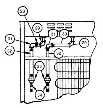
NOTE: Use pipe joint compound or Teflon tape on all threaded connections to assure a good water seal.
