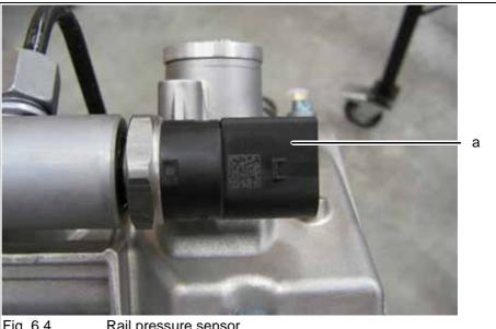
Fig. 6.4Rail pressure sensoraRail pressure sensor
