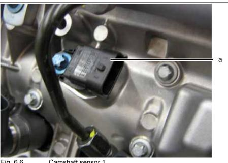
Fig. 6.6 Camshaft sensor 1 a Camshaft sensor FADEC A (1 of 2)
