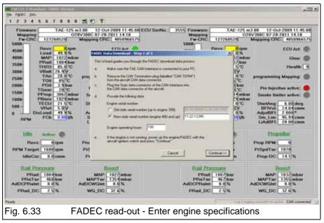
b) If not already active, establish CAN communication with the FADEC by following the steps on the screen. Enter the required engine S/N and engine run time. Select Continue. The following screen will appear:
