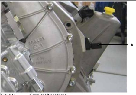
Fig. 6.9 Crankshaft sensor 2 a Crankshaft sensor FADEC B (2 of 2)
