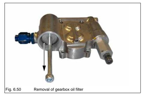
7. Insert the new gearbox oil filter. For mounting direction see Fig. 6.51 and Fig. 6.52.
