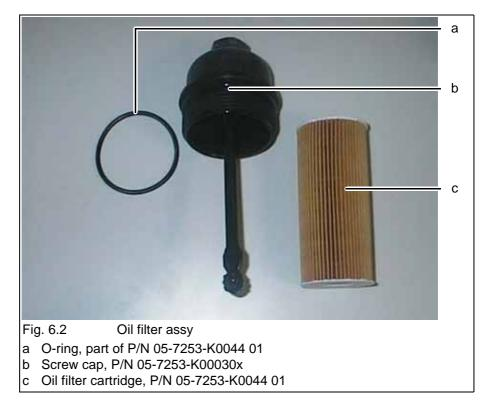
Refit the screw cap (b) and tighten it up to the specified tightening torque.
