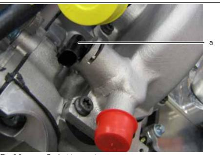
Fig. 6.3 Coolant temperature sensor a Coolant temperature sensor
