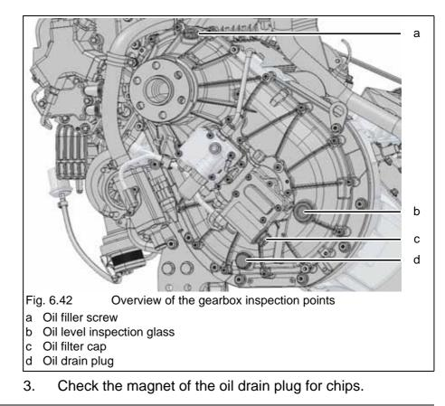
■ CAUTION: In case of any chips contact Technify Motors GmbH.
