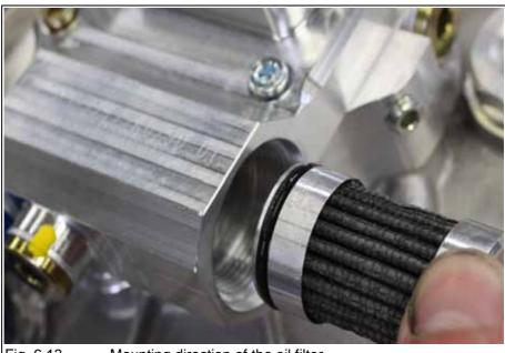
Fig. 6.13 Mounting direction of the oil filter
