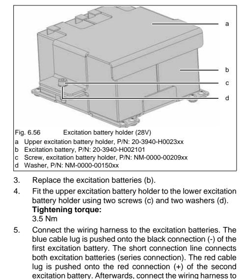
the wiring harness of the alternator regulator ("Exc. Batt"
