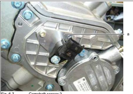
Fig. 6.7 Camshaft sensor 2 a Camshaft sensor 2 FADEC B (2 of 2)
