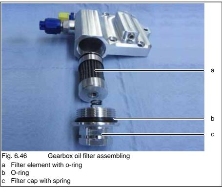
8. Attach the new o-ring to the filter cap. See Fig. 6.46.
