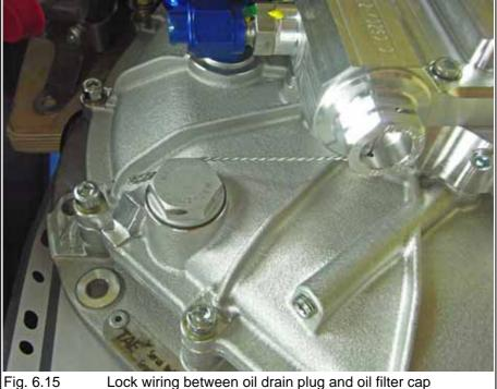
Lock wiring between oil drain plug and oil filter cap
