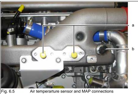
Air temperarture sensor and MAP connections of the intake manifold
