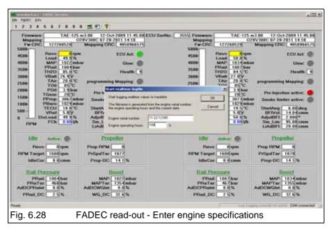
c) Enter the Engine S/N and Engine run time in the fields provided. Select OK. The window at the bottom right of the screen will indicate that the logging function is active by showing the file name in blue text.
