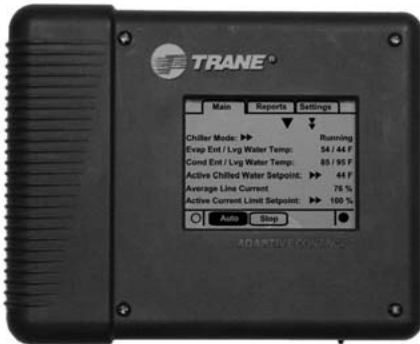
Figure 17. DynaView™ main processor
