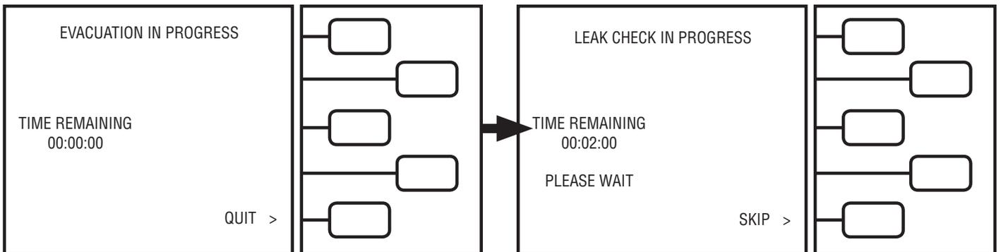
If leak check fails, check A/C system for leaks.
