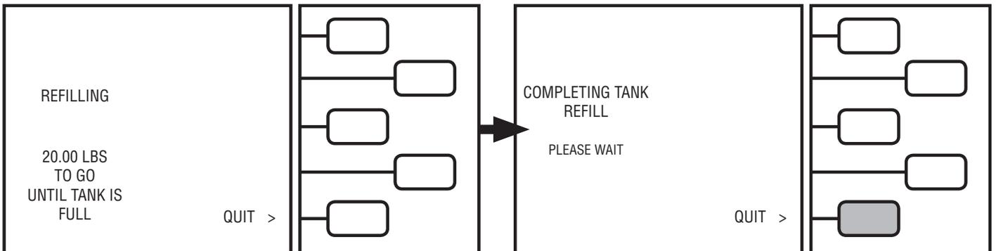
**The unit will run until: 1. REFILLING amount on LCD reaches zero or 2. Virgin supply tank is pulled into a vacuum**
