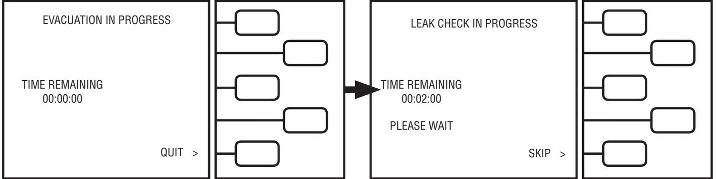
Once the **LEAK CHECK** has passed or the **SKIP** key is pushed, The LCD will read: Open the oil injection valve until the desired amount is dispensed. Push the **CONTINUE** key
