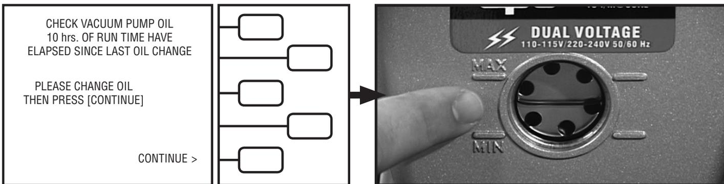
**Check Vacuum Pump Oil:** The oil level can be seen through the
