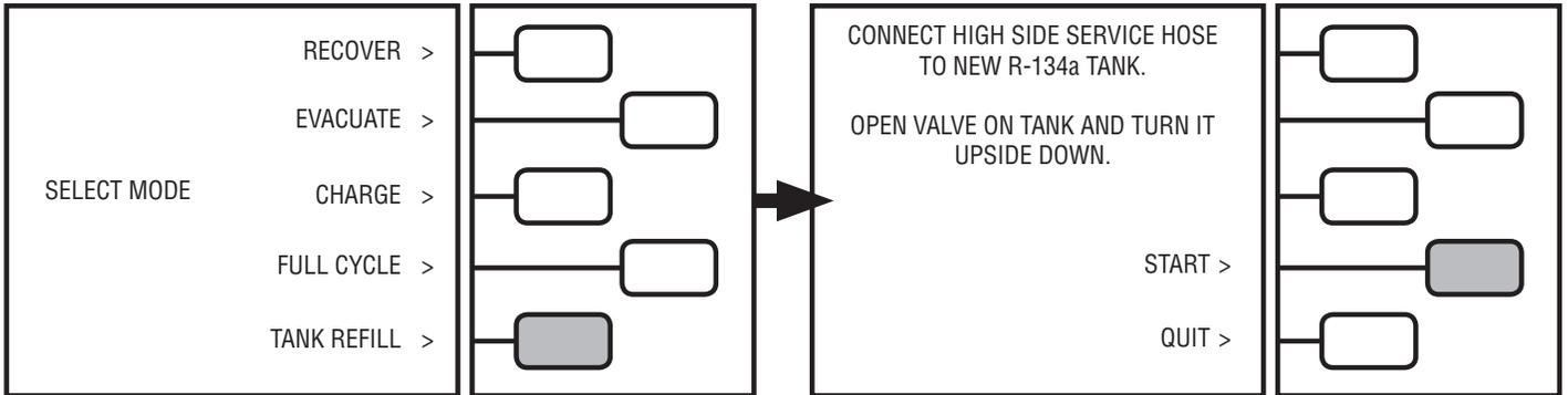
**Note: To speed up the Refill process, turn the supply tank upside down or make sure the liquid refrigerant is being recovered.**
