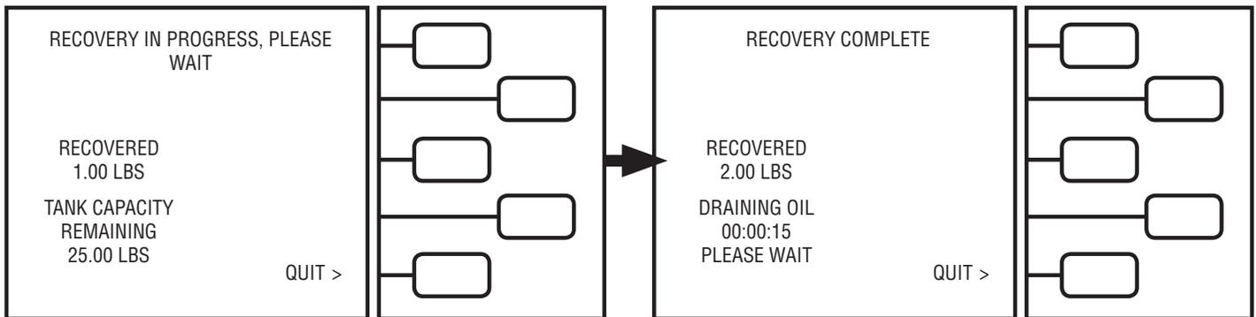
Record the **RECOVERED** weight reading on the LCD. Push the **QUIT** key to return to **Main Menu** (as shown below) or **PROCEED TO EVACUATE** key for evacuation operation. Do not forget to measure the A/C oil in the oil drain bottle for future A/C oil re-injection. **RECOVER/RECYCLE** Operation is now complete.
