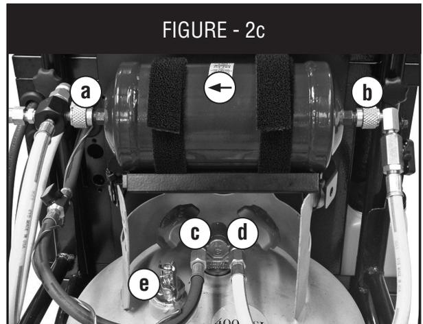
Hose routing between filter, tank, and unit
