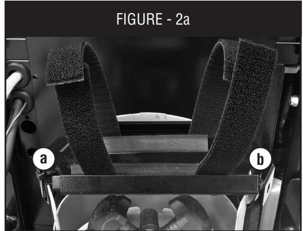
Filter bracket placed on tank collar
