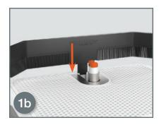
1 a-b Insert THE GUARD2 into slot
