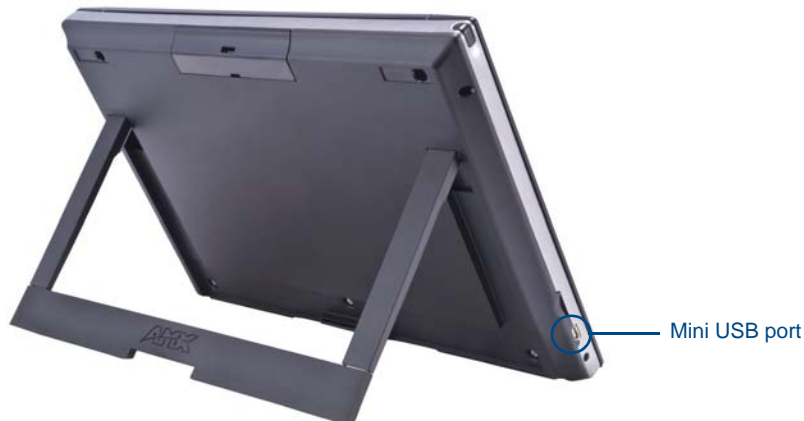
FIG. 31 USB Port on the MVP-9000i
