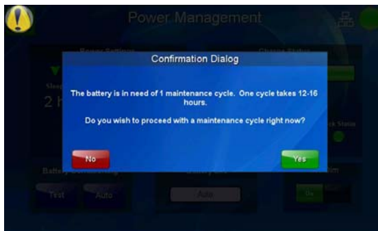
FIG. 58 Battery In Need of Maintenance Cycle popup window
