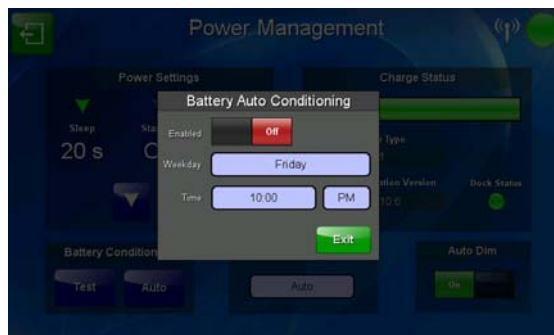
FIG. 55 Battery Auto Conditioning popup window
