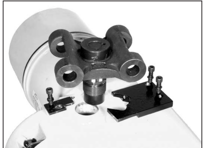
Figure 7-20. Removing Suspension Lug (1/4 through 1 Ton Models)
