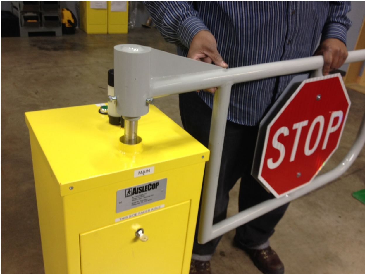
Figure 3. – Pedestrian Gate Arm Mounting
