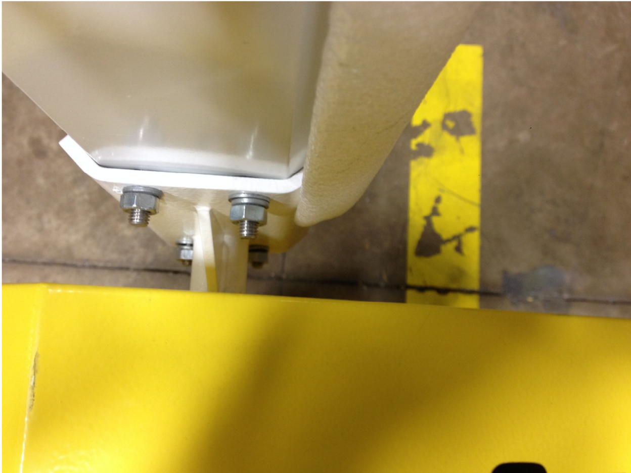
Figure 2. – Vehicle Gate Arm Mounting
