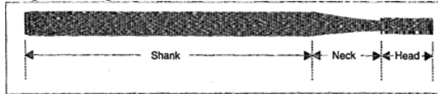
Figure (11): Normal designation of three parts of rotary cutting instruments.
