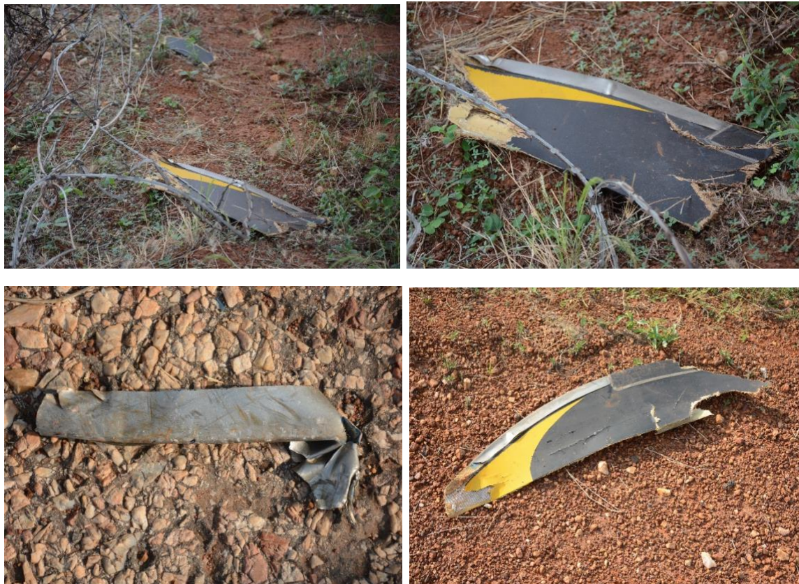
Figure 11: Debris of Damaged Propeller
