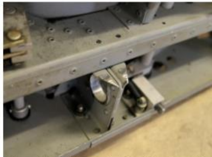
Figure 15 : Fretting on left fore/aft tube guide
