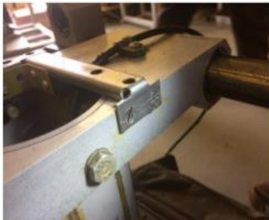
Figure 14 : Fretting on carrier assembly
