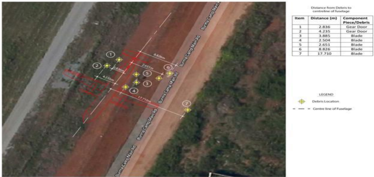
Figure 10: Aircraft impact debris distribution pattern
