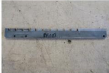
Figure 6 : Pre-mod side lock rail
