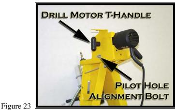
When re-installing, position the set screw through the mounting hole. Make sure that the motor's power cable is pointing toward the floor of the machine. Reinstall and tighten the T-knob.
