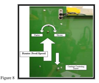
The Router Feed Rate Adjustment knob is located just under the air inlet port on the left side of the machine. (Figure 8) The adjustment knob only affects the cutting stroke of the pocket router. Turning the knob clockwise selects a slower Feed Rate. Turning the knob counter-clockwise selects a faster Feed Rate. A suggested Router Feed Rate Adjustment for hardwoods such as oak or maple is described as follows:
