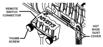
Figure 2-17 Remote Switch Installation
