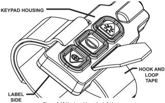
Figure 2-18 Hook and Loop Installation
