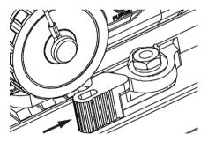
Figure 2-12 Throw Lever Mount Closed and Locked
