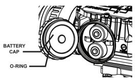
Figure 2-1 Battery Installation
