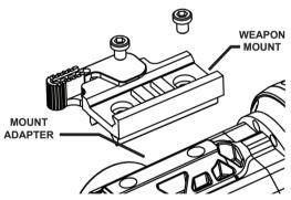
Figure 2-7 Weapon Mount Installation
