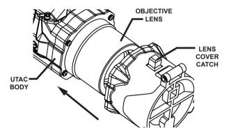
Figure 2-5 35mm Lens Cover Installation
