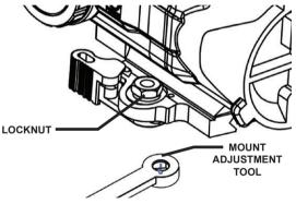
Figure 2-13 Locknut Adjustment
