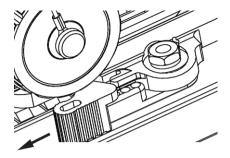
Figure 2-9 Slide Lock in Unlocked Position
