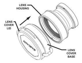
Figure 2-6 50mm Lens Cover Installation
