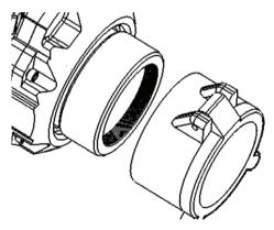
Figure 2-4 19mm Lens Cover Installation
