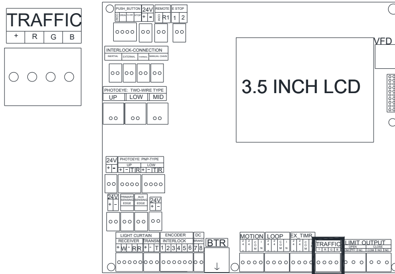
Figure 7.9. Audio Visual Warning Devices
