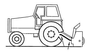
Equal Angles at Driveline Joints
