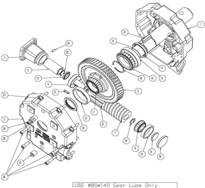
USE #85W140 Gear Lube Only. DO NOT use grease for lubricant.
