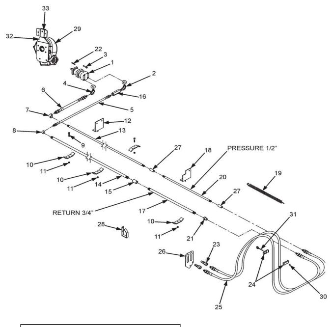
Truck Mounts: Pressure & Return Lines are Both 3/4"
