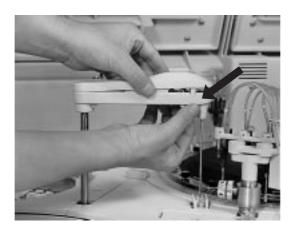
1. Remove the cover of the respective probe arm and disconnect the connection wires on the probe and serum tube. Make certain that the seal is not lost. Put it in a safe place.
