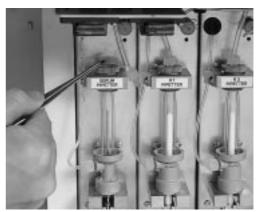
7. Refit the syringe with the glass body and the O-ring (L 456006 for sample/reagent syringes, 737-1629 for the ISE syringe) into the holder and tighten the knurled screw.
