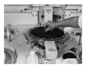
3. Loosen the retaining knob of the reaction disk and pull the disk up and out of the analyzer.
