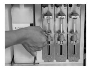
The sample syringe is situated behind the left front door. It is the first syringe to the right of the detergent bottles. Loosen the upper and lower tube connections by turning the retaining nuts in an anti-clockwise direction. Soak up any spilt water with an absorbent cloth.
