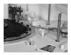
1. Loosen the two retaining screws opposite each other and pull the paddle down and out.
