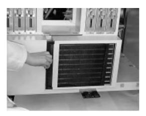
1. The air filter is situated behind the left front door of the analyzer. Open the door and remove the filter from its holder.
