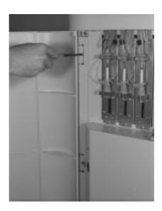
1. Remove the screws on the front of the analyzer as shown above and open the side door. Pull the rubber tube out of the vacuum tank.
