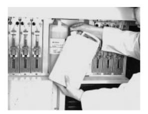
1. Place a new bottle with NaOH-D detergent in the position on the left. The position on the right is reserved for a second detergent. Make sure that the tube filter reaches the bottom of the bottle.
