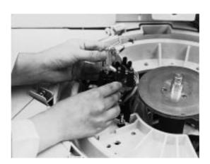
7. Fit the new lamp and reassemble the lamp in reverse order (as illustrated).
