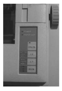
10. Press the FF switch (Form Feed) on the control panel of the printer. The print head will now move into its home-position. The paper will be automatically pulled into the print start-position by approx. 7mm.
