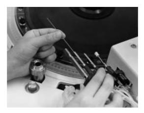
Pull all tubes off the cell rinse nozzle that is to be cleaned. Press the retaining clamp of the cell rinse nozzle and pull the retaining clamp and the cell rinse nozzle out of the cell rinse unit.
