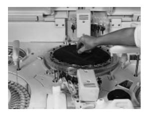
3. Loosen the retaining knob on the reaction disk and pull the disk up and out of the analyzer.
