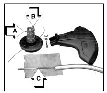
5. Install the bearing housing and shield.
