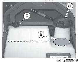
2. Fill the fuel tank until the fuel level reaches level point (b) at the base of the fuel tank opening. An expansion cavity above level point (b) is provided for proper operation of the venting port (c).
