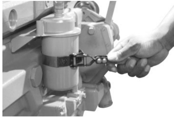
Changing Oil And Oil Filter Before First 100 Hours
