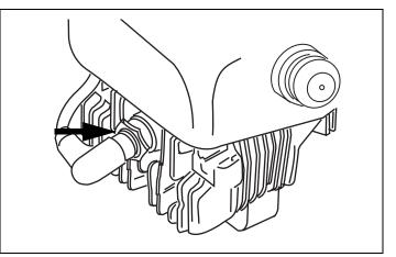
Figure 17. Typical Spark Plug Connection
