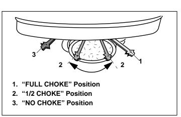
Figure 12. Choke Control "B"
