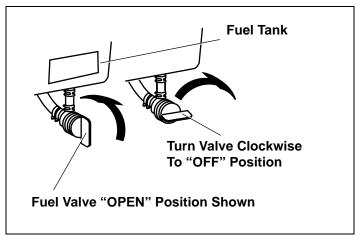
Figure 8. Fuel Valve Positions
