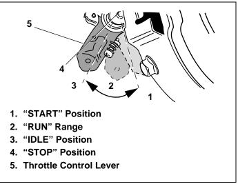
Figure 10. Remote Throttle Control
