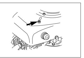
Figure 6. ON/OFF Switch
