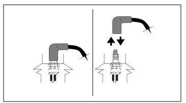
Figure 1. Disconnecting/Connecting Spark Plug
