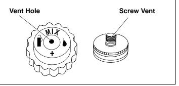
Figure 7. Fuel Cap Vent Hole and Optional Screw Vent
