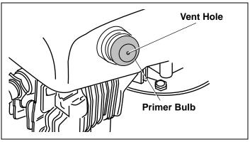
Figure 13. Engine Primer Bulb
