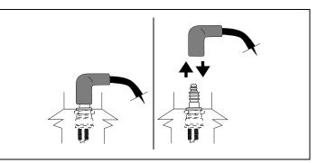
Figure 16. Disconnecting/Connecting Spark Plug
