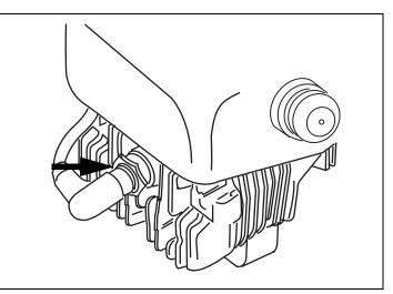
**Figure 2. Typical Spark Plug Connection**
