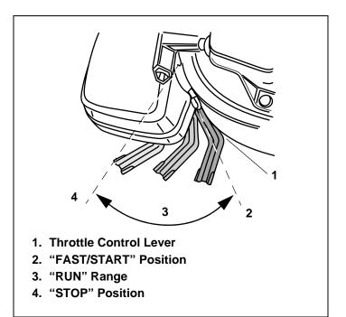
Figure 15. Variable Speed Engine Control
