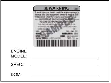
Figure 3. Engine Identification Decal
