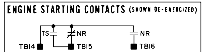
Figure 1-3. Engine starting contact label and location for 30, 70 and 104 amp. B-design transfer switches and 150 and 200 amp. C-design transfer switches.
