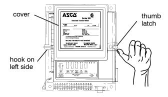
Figure 4-1. Controller cover latch.
