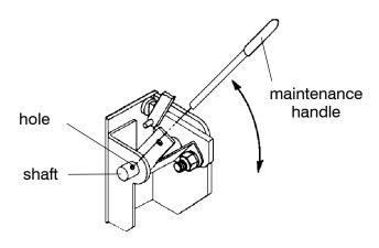
Figure 1-4. Removable maintenance handle on 260 and 400 amp. E-design transfer switches.
