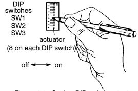
Figure 4-4. Setting DIP switch actuators.
