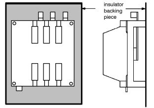
Figure 1-1. Insulator for 260 and 400 amp. E-design transfer switches.
