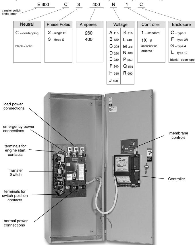
400 amp. size in typical enclosure with location of customer connections
