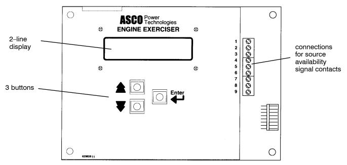
Figure 5–2. Accessory 11BG module (mounted behind operator interface and connected to the controller) includes source availability signal contacts and a programmable engine exerciser.
