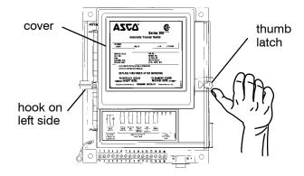
Figure 4-1. Controller cover latch.
