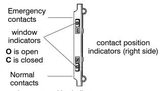
Figure 1-4. Maintenance handle operation and contact position indicators.
