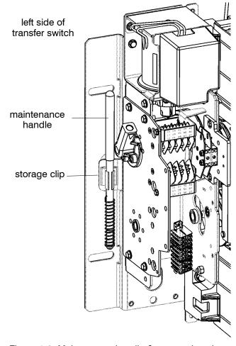
Figure 1-3. Maintenance handle & storage location.
