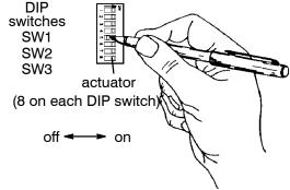
Figure 4-4. Setting DIP switch actuators.
