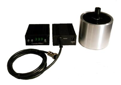
The Condor Power Supply Unit (PSU) is a microprocessor controlled digital regenerative AC power source used for accurate speed control of a turntable motor. The PSU uses Direct Digital Synthesis (DDS) to create an extremely accurate and clean sine wave that improves motor speed stability and allows the user to precisely adjust the turntable platter rotational speed.
