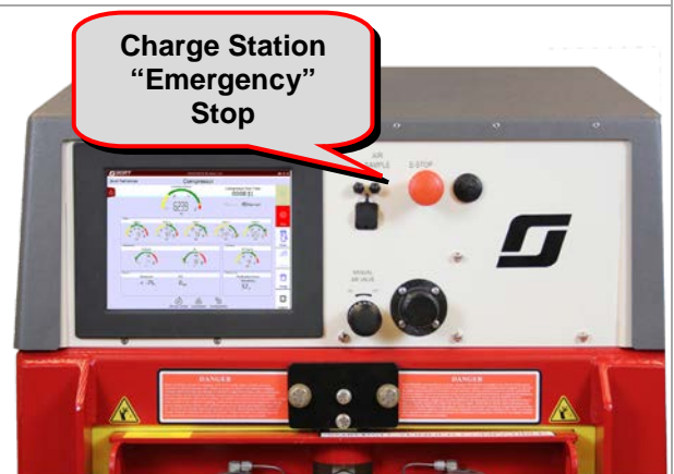
Figure 3.4-3: Charge Station Emergency Stop
