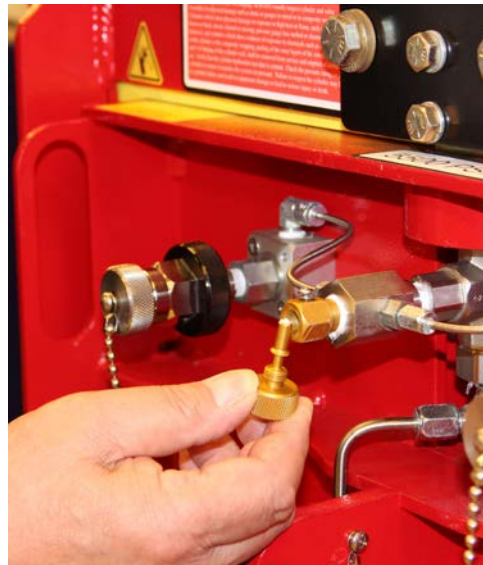
Figure 4.8-2: Remove Bleeder Knob
