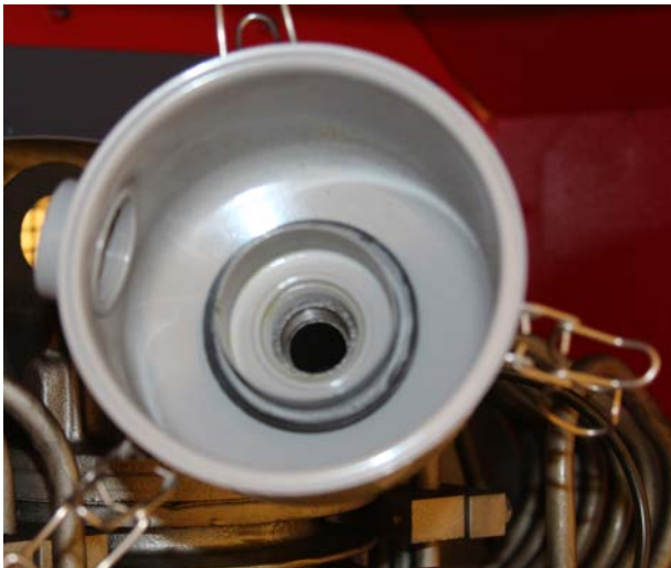
Figure 4.6-7: Intake Filter Housing
