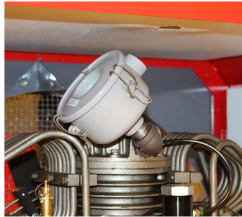
Figure 4.6-2: Intake Filter Location
