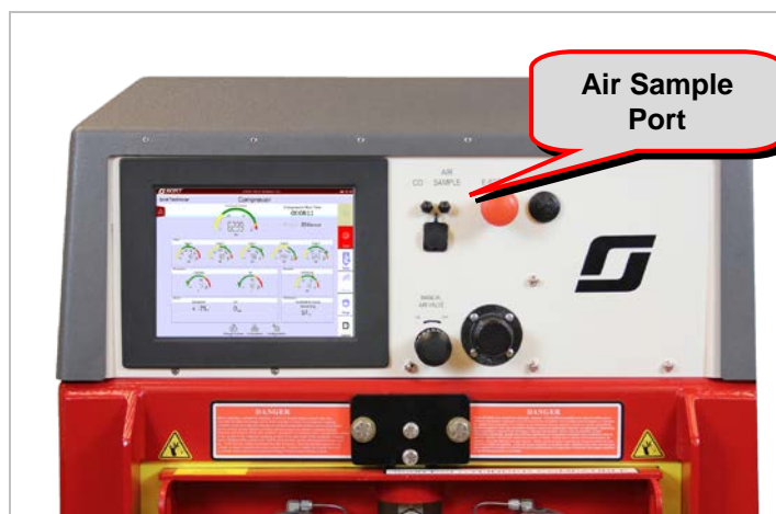
Figure 4.3-1: Air Sample Port
