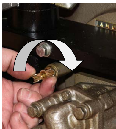
Figure 4.5-15: Close Crankcase petcock
