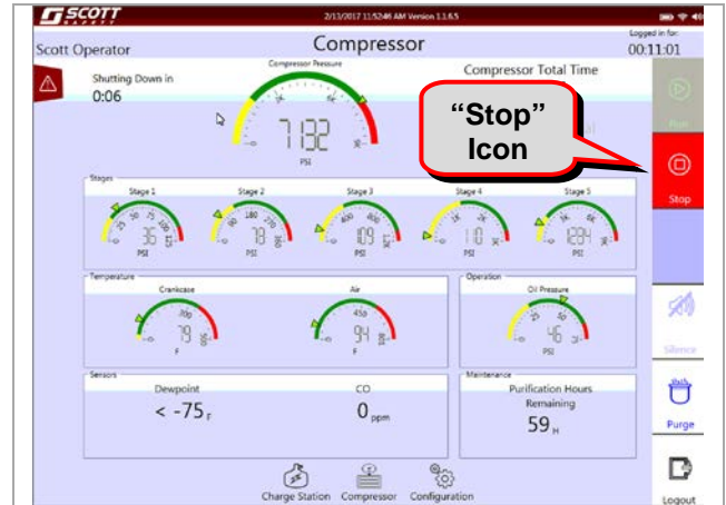
Figure 3.4-1: Compressor Shut Down
