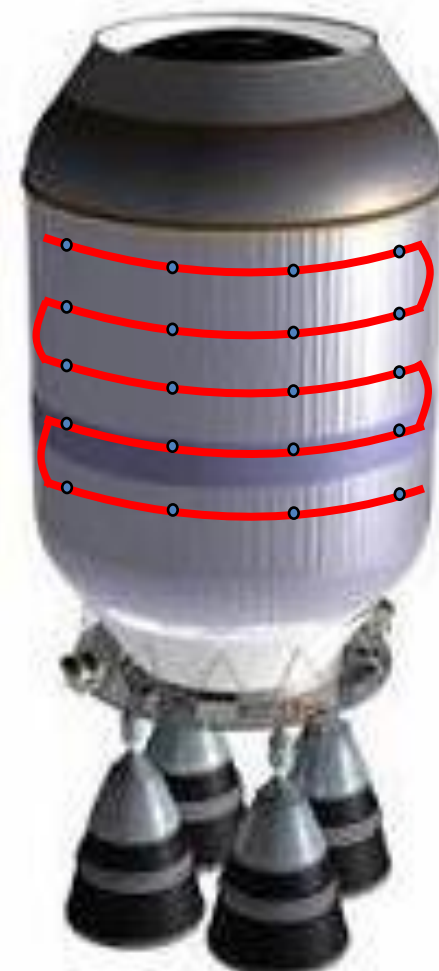
Example hyFOSS fiber layout
