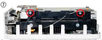
Once you have removed the 2 screws on the right side, rotate the Mac mini 180 degrees and remove the 2 Phillips screws circled above from the optical drive on this side.
