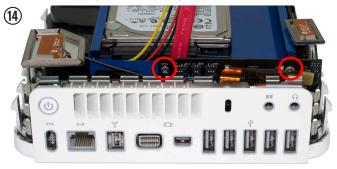
Turn the Mac mini around so that you can see the rear ports. Insert the remaining 2 Phillips screws you removed from the optical drive into the OWC Data Doubler, again being careful of the copper-colored ribbon cable you disconnected to gain access to the concealed Phillips screw.
