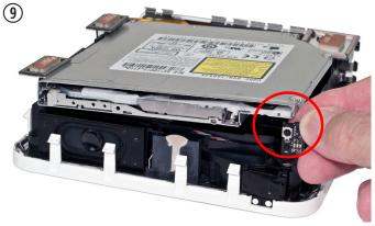
Turn the Mac mini around to the front so that you can see the slot in the optical drive.
