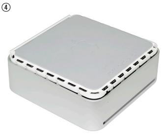
All of the plastic retaining clips must be released as described in step  $\$  before the top cover will separate from the bottom housing.
