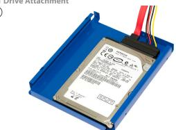
Take the SATA cable that came bundled with your OWC Data Doubler and insert the large end of the SATA plug onto the hard drive that you are going to install into the bracket. It will only fit one direction, and it is keyed to prevent improper installation. Once that is inserted, gently set the hard drive into the OWC Data Doubler bracket with the SATA cable towards the back of the OWC Data Doubler, as shown in the above picture.
