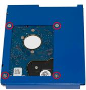
While holding the drive in the bracket, turn the OWC Data Doubler over so that you can see the bottom. Insert the 4 included Phillips screws through he bracket, into the bottom of the hard drive. Insert the first screw a few turns and then start the other screws before fully tightening all of them.
