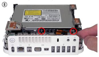
Turn the Mac mini around so you can access the rear of the computer. There are two remaining screws holding the optical drive into the Mac mini.
