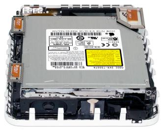
Once you have removed the top cover of the Mac mini, you can see the plastic clips that are snapped into the top cover.
