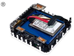
Place the OWC Data Doubler into the Mac mini from the front and slide it all the way into the Mac mini chassis.
