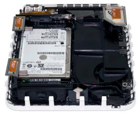
Once you have removed the optical drive, you can see where you are going to install the OWC Data Doubler into the Mac mini.
