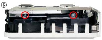
Looking at the front of the Mac mini, turn it so that you can see it's right side. Remove the 2 Phillips screws that are circled above from the optical drive.
