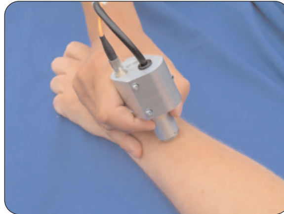
Figure IV – Photograph of the handheld scanning probe in use imaging a volunteer's arm.
