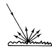
Figure 1.9 Scattering from a rough surface
