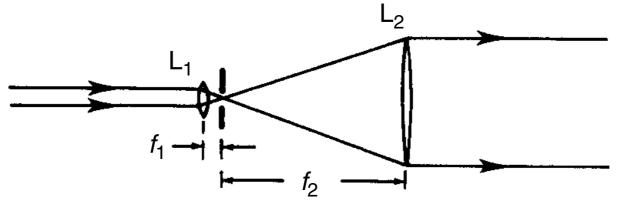
Figure 1.14 A plane wave set-up
