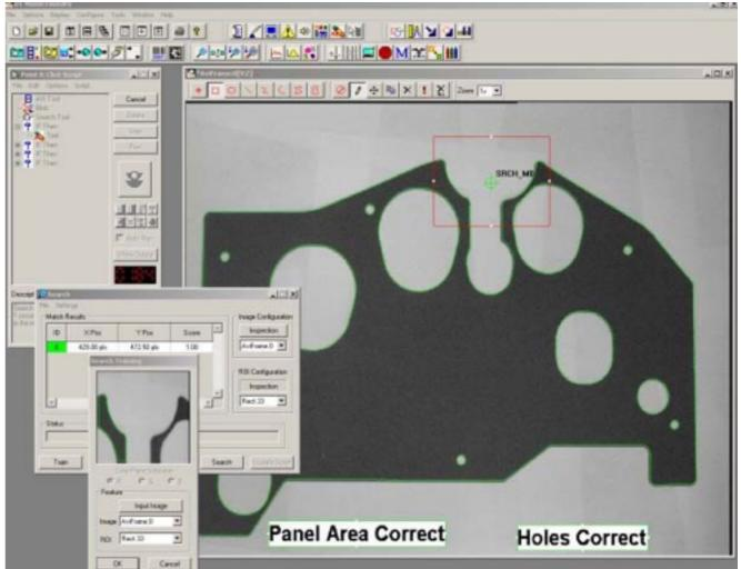
Vision-Based Metrology inspection systems evolved from the combination of microscopes, cameras and optical comparators.
