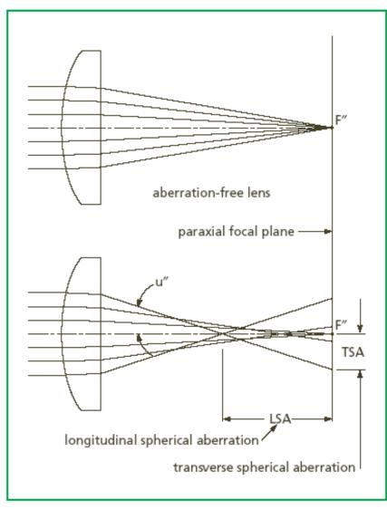
Spherical aberration of a plano-convex lens
