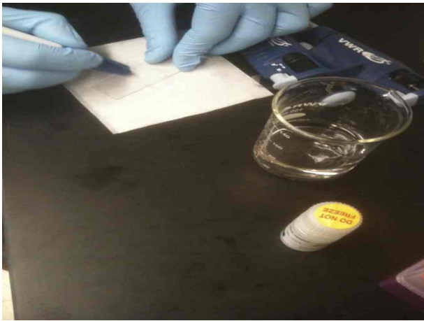
FIG. 21. Image detailing the use of a marker cap to press the coverslip to the double-sided tape and slide.
