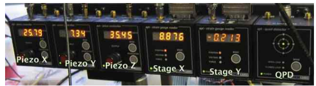
FIG. 8. Photograph of the stage position and quadrant photodetector displays on the T-cube blocks.
