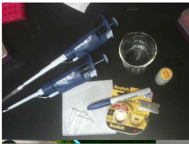
FIG. 16. Image of the useful materials for preparing a free-floating bead sample.
