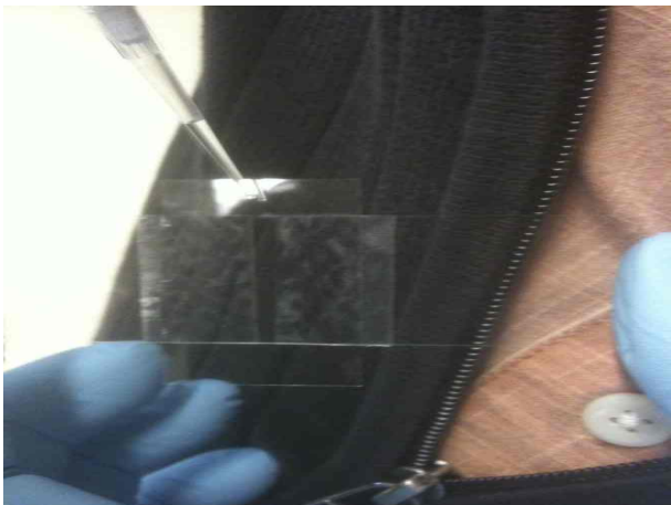
FIG. 22. Injecting bead solution into the channel.
