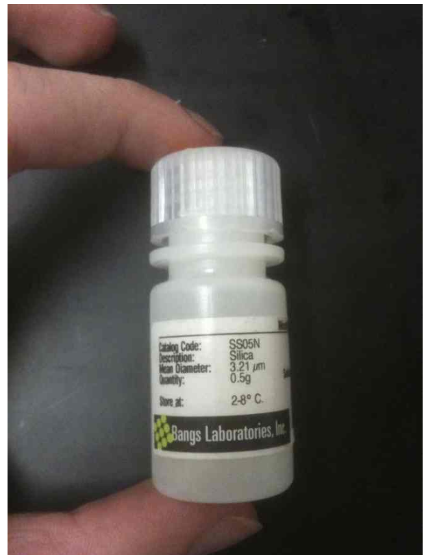
FIG. 12. Stock solution of silica microspheres.
