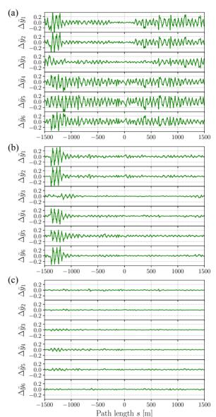
Figure 7: Measured vertical leakage orbits induced by horizontal dipole kicks in the LER ring (a) before correction, (b) after correction, (c) after two countermeasures for the leakage field of the Lambertson septum magnet. The vertical axis is normalized by root-mean-square amplitudes of the horizontal orbit.
