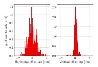
Figure 6: Offset distribution for the LER BPMs.
