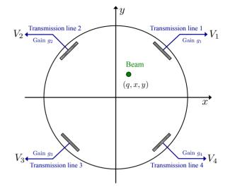
Figure 1: Schematic view of the BPM model used in BGC.
