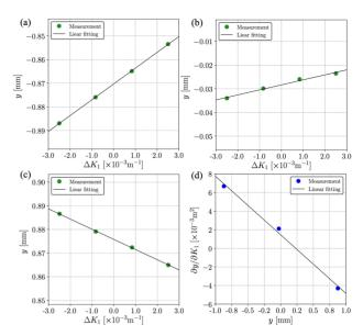
Figure 5: Example of BBA. Beam positions y as a function of the field gradient of adjoined quadrupole magnet  $K_1$  for three kinds of closed orbits are shown in (a), (b) and (c). Orbit response  $\partial y / \partial K_1$  as a function of the BPM reading is shown in (d).
