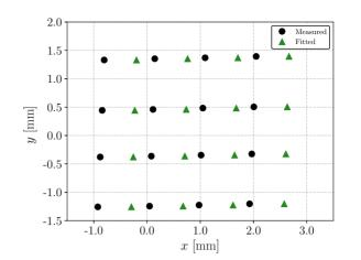
Figure 2: Example of the gain calibration. The dots represent measured beam position before the fitting, while the triangles represent beam positions obtained by the chi-square minimization.
