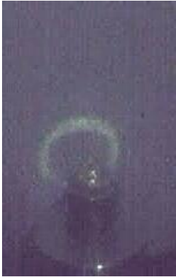
Figure 60: SHG ring in strontium barium niobate. The fundamental laser beam is directed along the crystallographic c -axis. In this direction, no SHG light is visible, instead a circular cone of green light is visible. The image shown corresponds to the second image of Fig. 57, the infrared light is suppressed by an appropriate filter.
