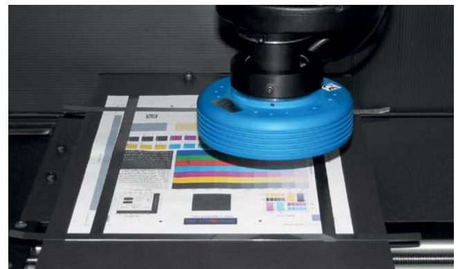
Fig. 35: A bi-telecentric lens is interfaced with a tunable filter in order to perform high resolution colour measurements. The image-side telecentricity ensures that the optical bandpass is homogeneous over the entire filter surface and delivers an even illumination of the detector, provided the object is evenly illuminated too.
