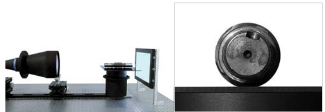
Fig. 34: Image of a thick object viewed throughout its entire depth by a bi-telecentric lens
