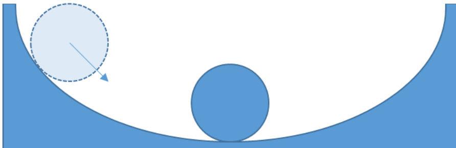
Fig. 1.1. Minimum total potential energy principle [own source]
