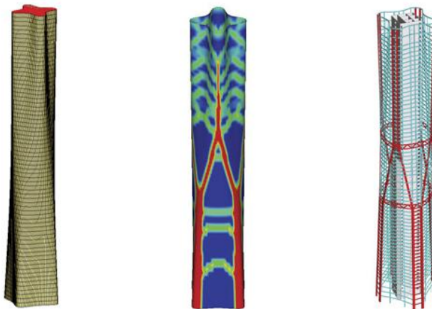
Fig. 4.3. Structure optimisation with the use of OptiStruct [5]
