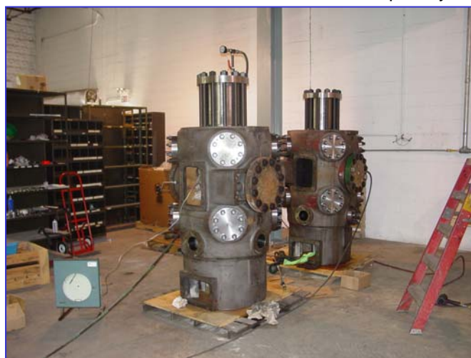
Fig. 23: Remanufactured cylinders with new fixed volume clearance pocket heads and valve caps undergoing an 8-hr factory hydrostatic test
