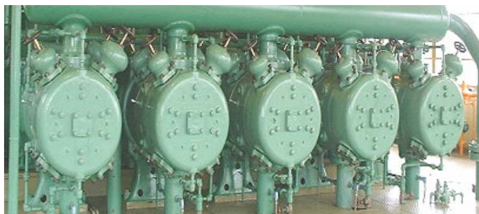
Fig. 33: One of five large 19.0 in. (483 mm) stroke integral engine compressors that were completely configured for automatic operation with a broad range of pressure ratios.
