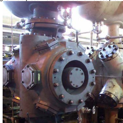
Fig. 10: New 18.125 in. (460.4 mm) bolt-in 2 nd stage replacement cylinder.
