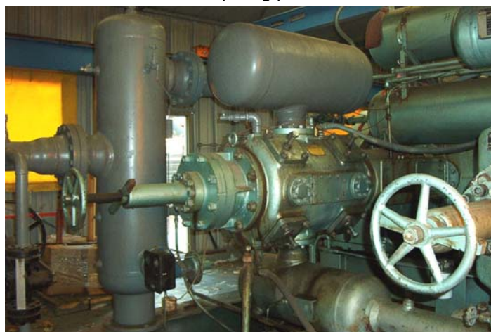
Fig. 36: With only manual control, this 2-stage Ajax compressor was either under-loaded or subject to frequent shutdowns to avoid overload.
