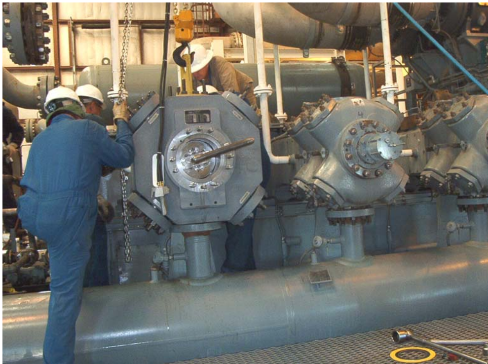
Fig. 12: The first of six new high efficiency bolt-in replacement cylinders [left] is installed on a six-throw, single-stage D-R 6HOS-6 frame. Two of the original OEM cylinders are shown on adjacent throws [right] prior to replacement.
