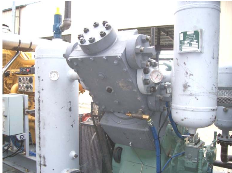
Fig. 20: 2500 psig (172.4 bar) cylinder family developed to fill a gap in the OEM's offerings for high-pressure air drilling service.
