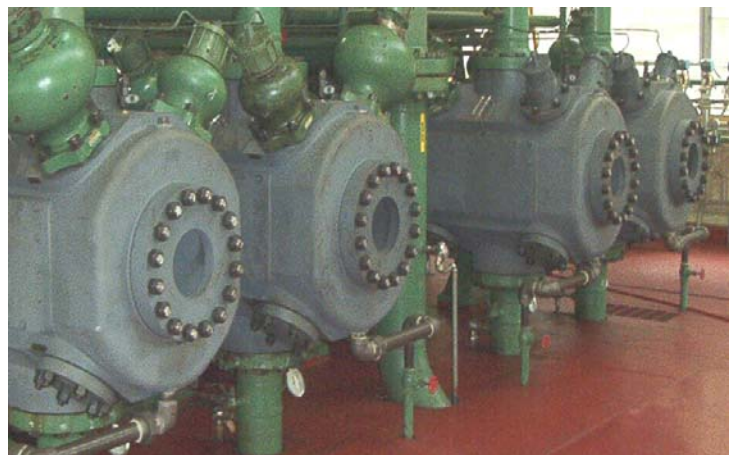
Fig. 14: New custom engineered 1200 psig (82.7 bar) bolt-in replacement valve-in-barrel type cylinders.
