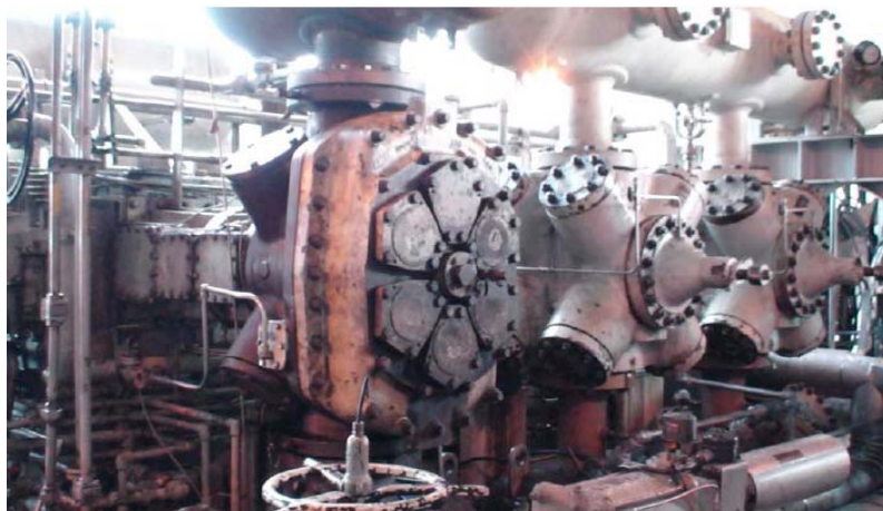
Fig. 9: Original 18.0 in. (457.2 mm) OEM 2 nd stage cylinder [left] that experienced frequent rapid, catastrophic piston failures due to a mis-application..
