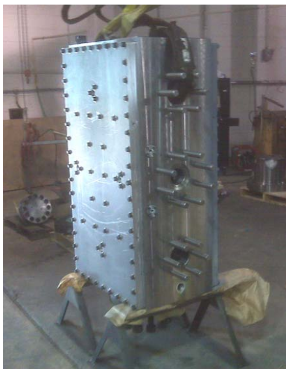
Fig. 6: New AISI 4140 forged steel cylinder with water jacket, weighing more than 10,000 lb. (4335 kg).
