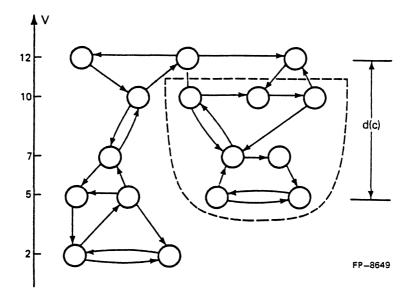
Fig. 2. A cup C is enclosed with dashed lines.  $\underline{V}(C) = 5$ ,  $\overline{V}(C) = 12$ , and d(C) = 7 and the bottom B of C contains two states.
