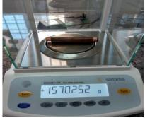
Fig. 11 Measuring the weight of the tool with the help of Semi Micro Balance
