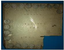
Fig.4 INCONEL-825 (after machining without heat treated and with heat treated)
