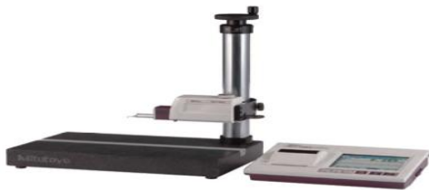
Fig 3. Surface roughness tester Mititoyo SJ-400
