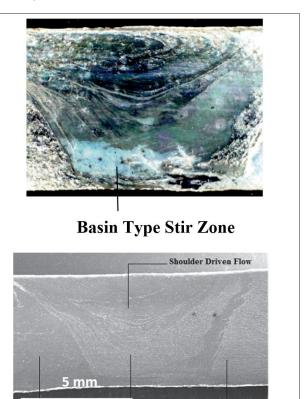
HAZ of Pin Driven Flow HAZ of ZM 21 AZ 31
