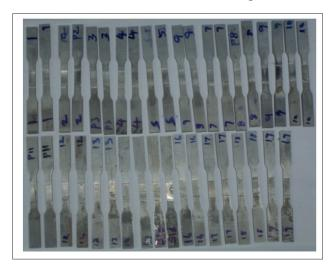
Fig. 3 - Photograph of EDM Wire Cut Tensile Samples
